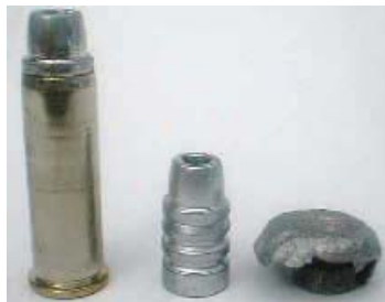
The 358446 HP, loaded into the .38 Special and similar bullet recovered after being fired into water at 1000 fps.
