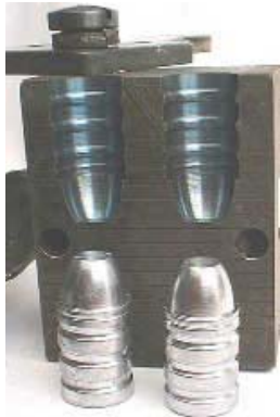
The Ideal 358443; the first bullet Lyman designed for the .357 Magnum.
