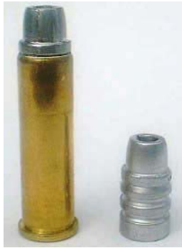
Lyman 358446 HP loaded into .357 Magnum cartridge.
