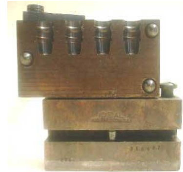
Ideal 4-cavity 358477 mould.
