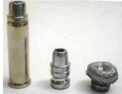
.38 Special and 358477 HP; loaded round, as-cast bullet, and bullet recovered after being fired into water at 1000 fps.
